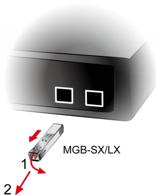
Figure 2-17: How to Pull Out the SFP/SFP+ Transceiver
